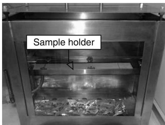
**Figure 1** Flame chamber used in this study with horizontal position for samples.
